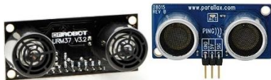
Figure 2: Photos of the URM37 (left) and PING (right) ultrasound sensors used in this project
