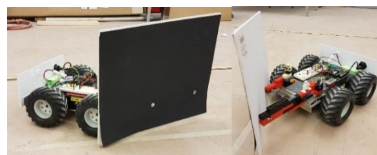
Figure 22: Photos of the target mounted on a Lynxbot robot car
